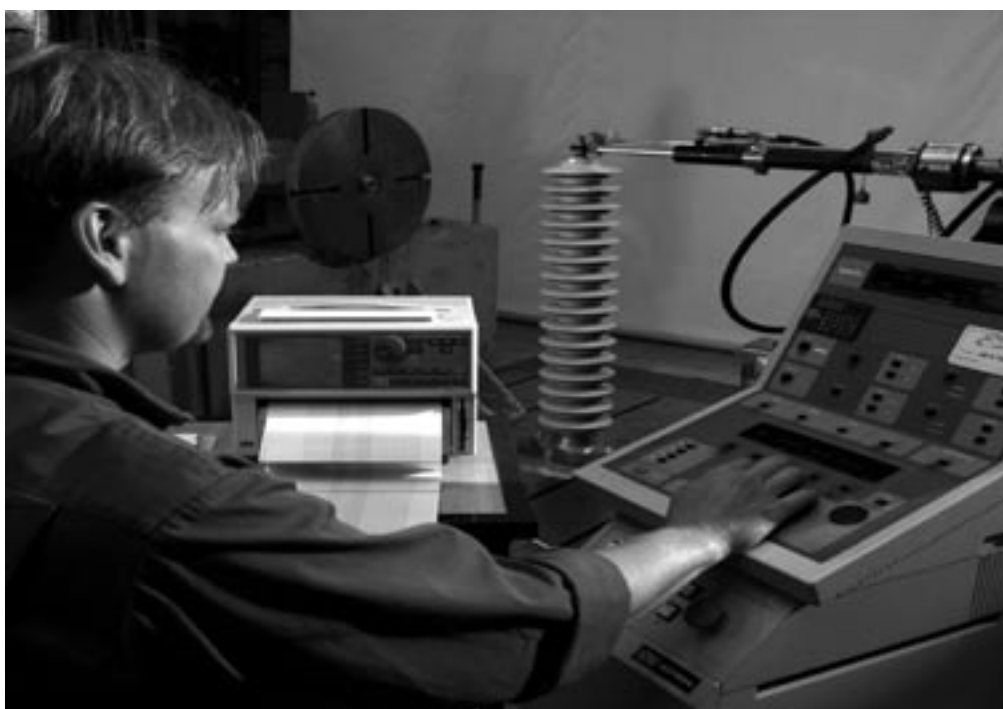
Mechanical test of silicone-housed arrester PEXLIM P.
